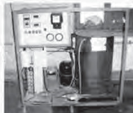
Vapour compression refrigeration test rig
